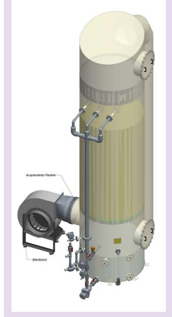
The gas flow, driven by the fan, passes through a layer of absorbent filler (Pall rings), receives a rain of water through the diffusers, to reach a droplet separator. The gas, already humidified, crosses a large pipe to the biomass bed.
